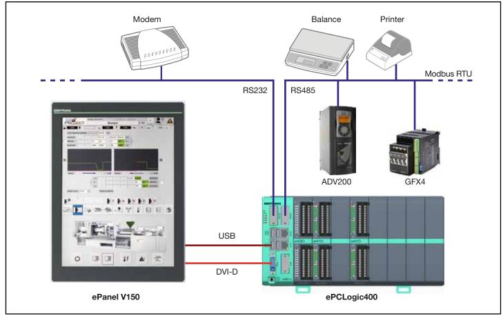
RS485 / RS232 - Modbus RTU System architecture
