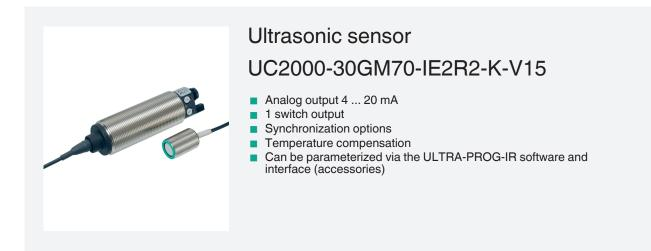
Ultrasonic diffuse sensor with separate transducer
