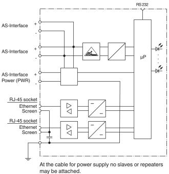
At the cable for AS-Interface circuit no power supplies or further masters may be attached.
