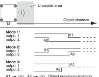
A1  $\rightarrow \infty$ , A2  $\rightarrow \infty$ : Object presence detection. Both outputs operate according to the selected mode, if an object is located within the detection range.
